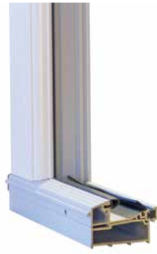
Stormguard Plus Threshold Distance from bottom of door leaf to bottom of threshold - 38mm. Available in Silver only.
